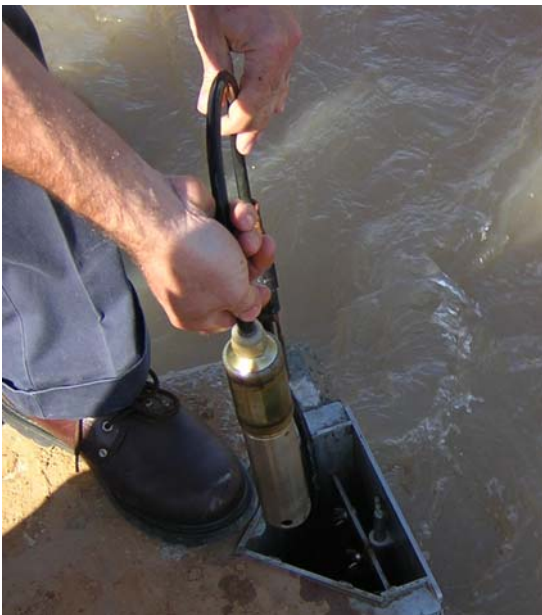
Figure 7.1-8: A Stage Logger being taken out of its Chamber
