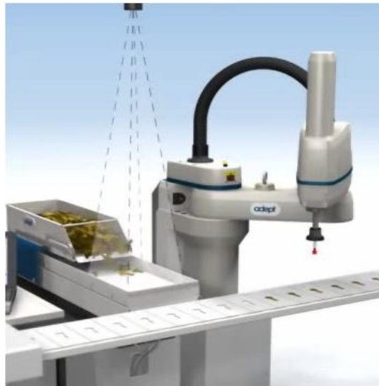
Figure 2.3: Adept Anyfeeder™ system representation (Adept, 2008),
