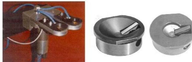
Figure 5.9: Dual automatic electrode dresser with removable cutter units (Rotech, 2001)
