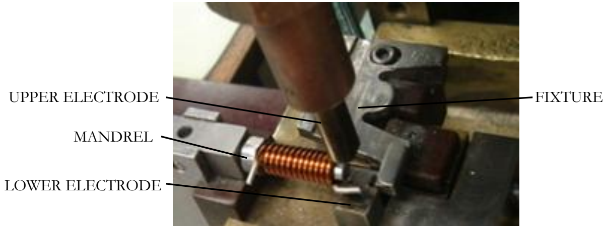
Figure 3.6: Mandrel weld fixture for coil alignment to handle frame assembly
