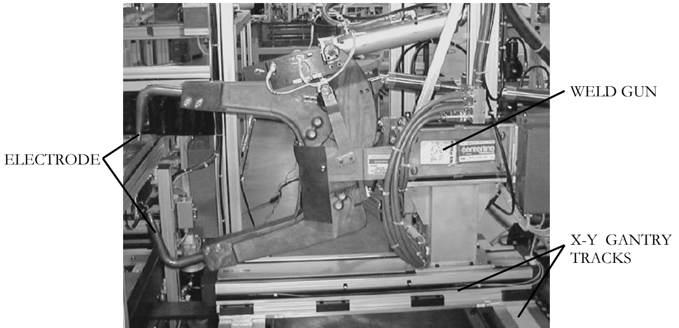
Figure 2.13: Robotic weld gun mounted on X-Y gantry (Bloss, 2006)
