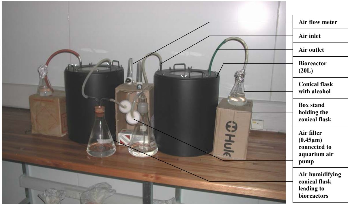
Figure 2: Twenty-litre bioreactors with FCCI unextracted wood chip samples incubated at 29 0 C for four weeks.
