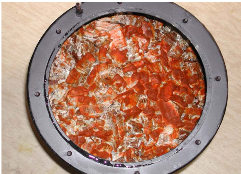
Figure 3: Top view of a twenty-litre bioreactor containing wood chips inoculated with fungal co-culture after incubation at 29 0 C for four weeks.
