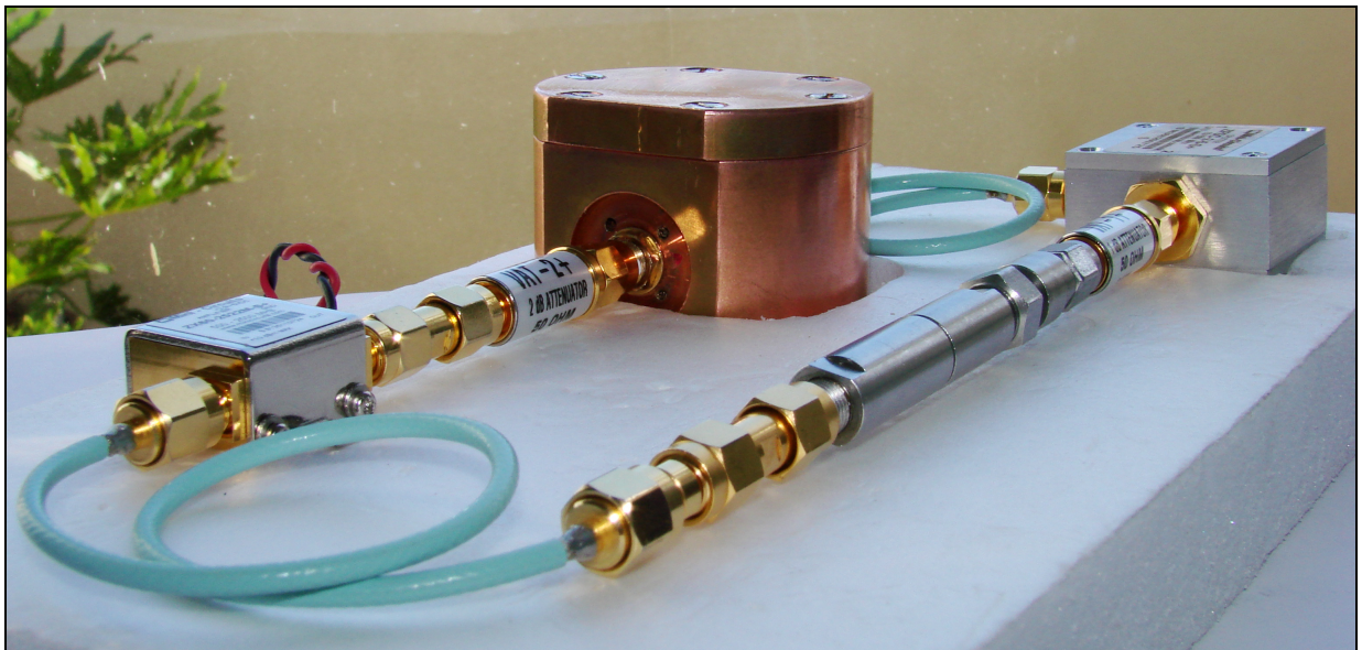
Figure 4.1: Photograph of the Voltage Controlled Oscillator System as a whole.
