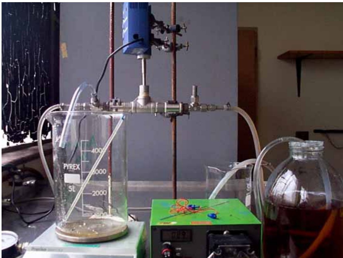
Figure B-4. Lab-scale setup showing permeate collection and measurement via scale.
