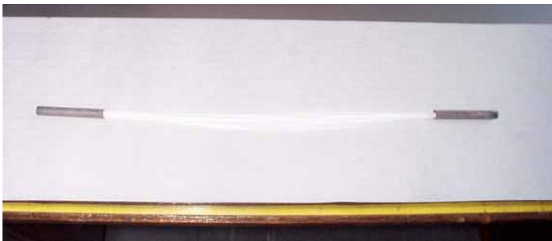
Figure B-2. The capillary ultrafiltration membranes – ends were epoxied into the 10 mm stainless steel tubing
