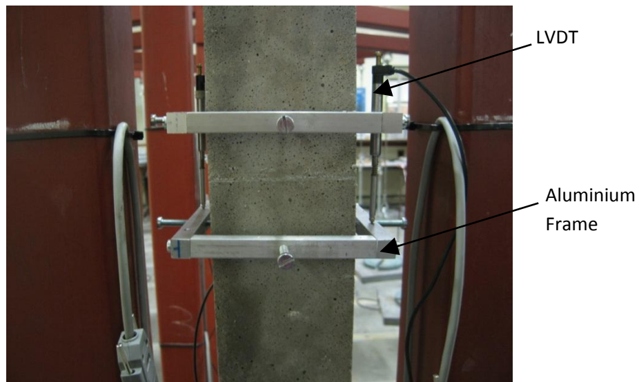
Figure 31 An example of the LVDTs and aluminium frames used.
