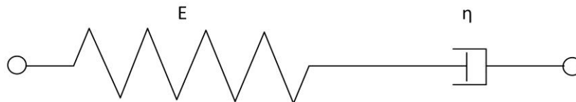
Figure 8 Graphical presentation of a spring-dashpot system. (Aklonis, 1981; Bower, 2002)
