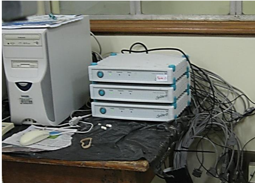
Figure 30 The Spider8 data loggers used in the experiments.
