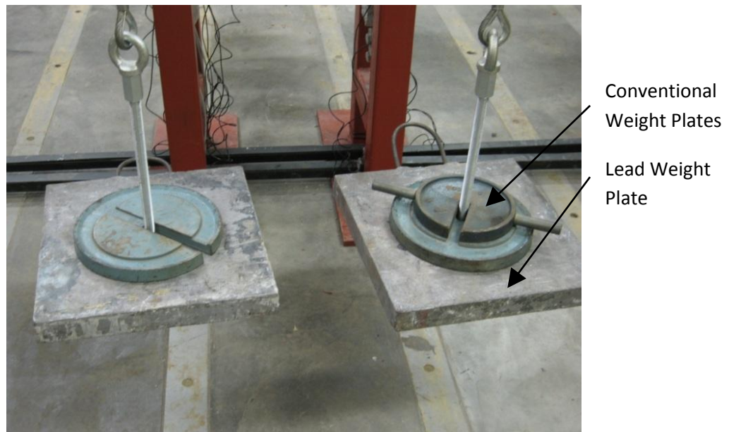
Figure 29 The loading was executed by weight plates.
