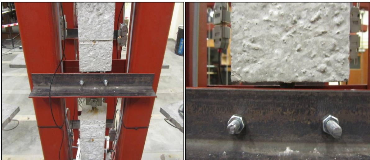
Figure 32 The secondary safety mechanisms a) Fitted to the frames with a spacing of b) more of less 5 mm.
