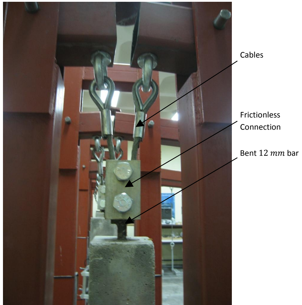
Figure 19 Figure demonstrating the interaction between the cables, connection and concrete specimen.
