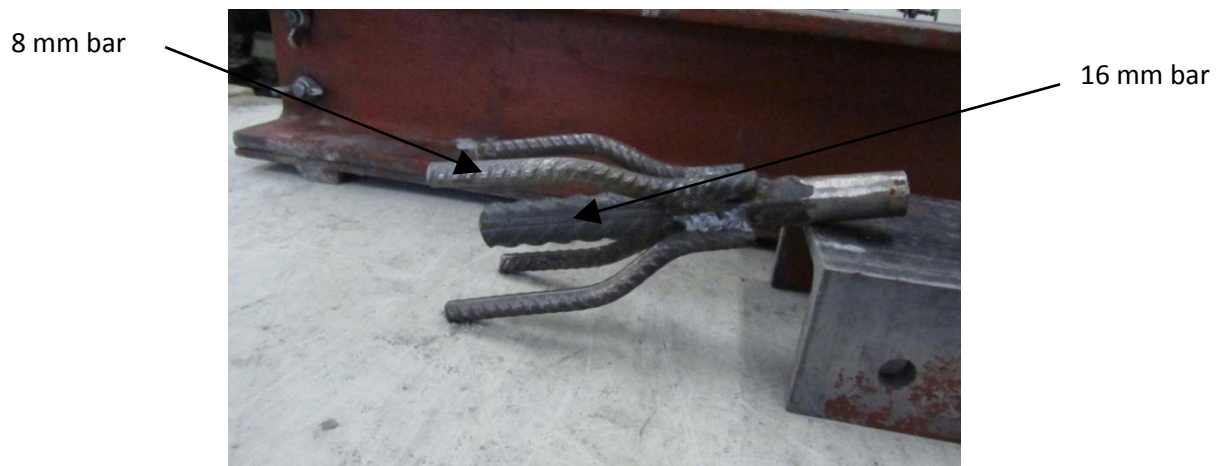
Figure 17 Steel hook specially modified for tensile strength tests.
