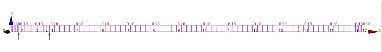
Figure 88 Supports and point load modelled on the pivot beam. (Prokon)
