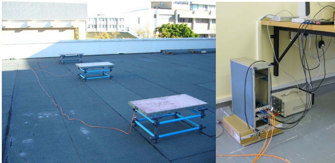
Figure 8.18: (a) Sensors with transmitters inside Faraday cage and (b) receivers inside Room E360.
