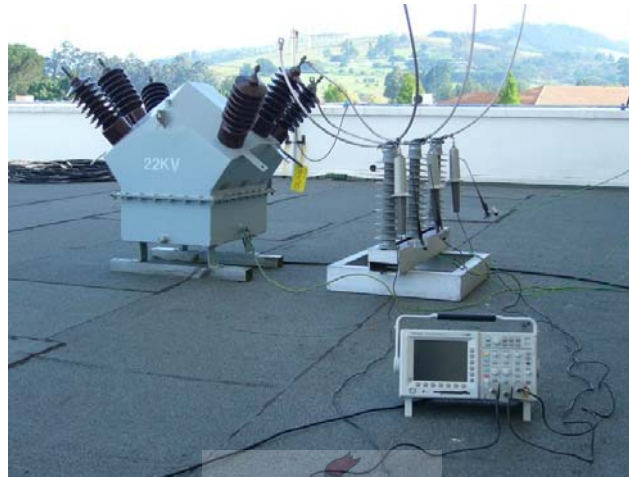
Figure 8.39: Test setup for measuring HV waveforms
