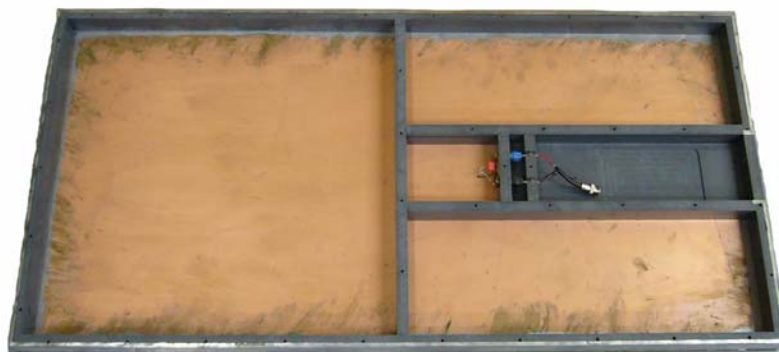
Figure 4.4: Photograph of the inside of Faraday cage and drawer, with the top plate of sensor assembly removed.
