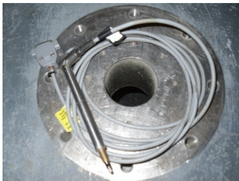
Figure 8: LVDT - Linear Variable Displacement Transducer
