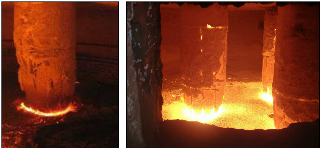
Figures 2.3.3 Photos of the furnace interior (a) Immersed electrode (b) Electrodes slightly raised.
