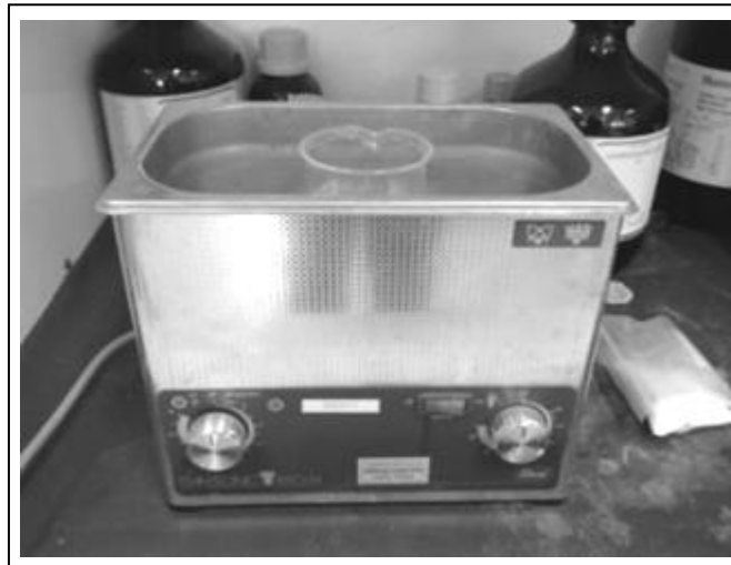
Figure 3.6: Experimental setup for ultrasound treatment of hemicelluloses
