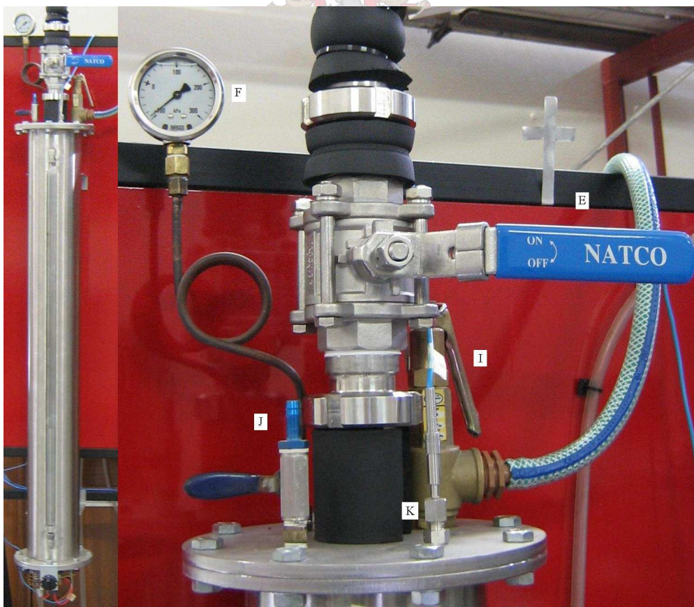
Figure 2.6: The uninsulated boiler (insert right: boiler top enlarged)
