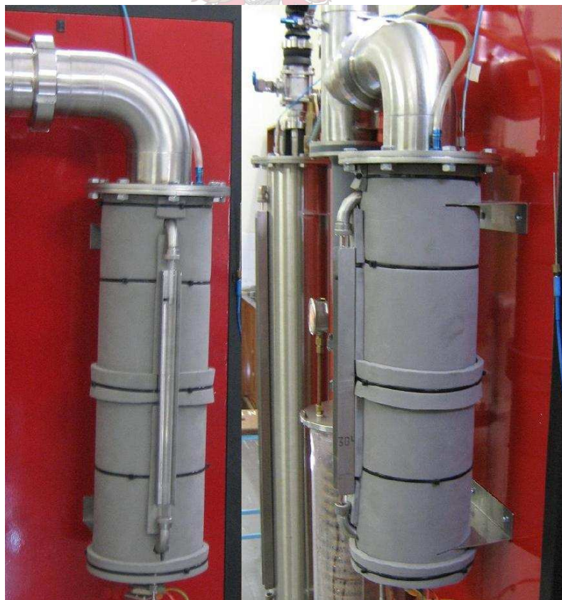
Figure 2.7: Partly insulated evaporator
