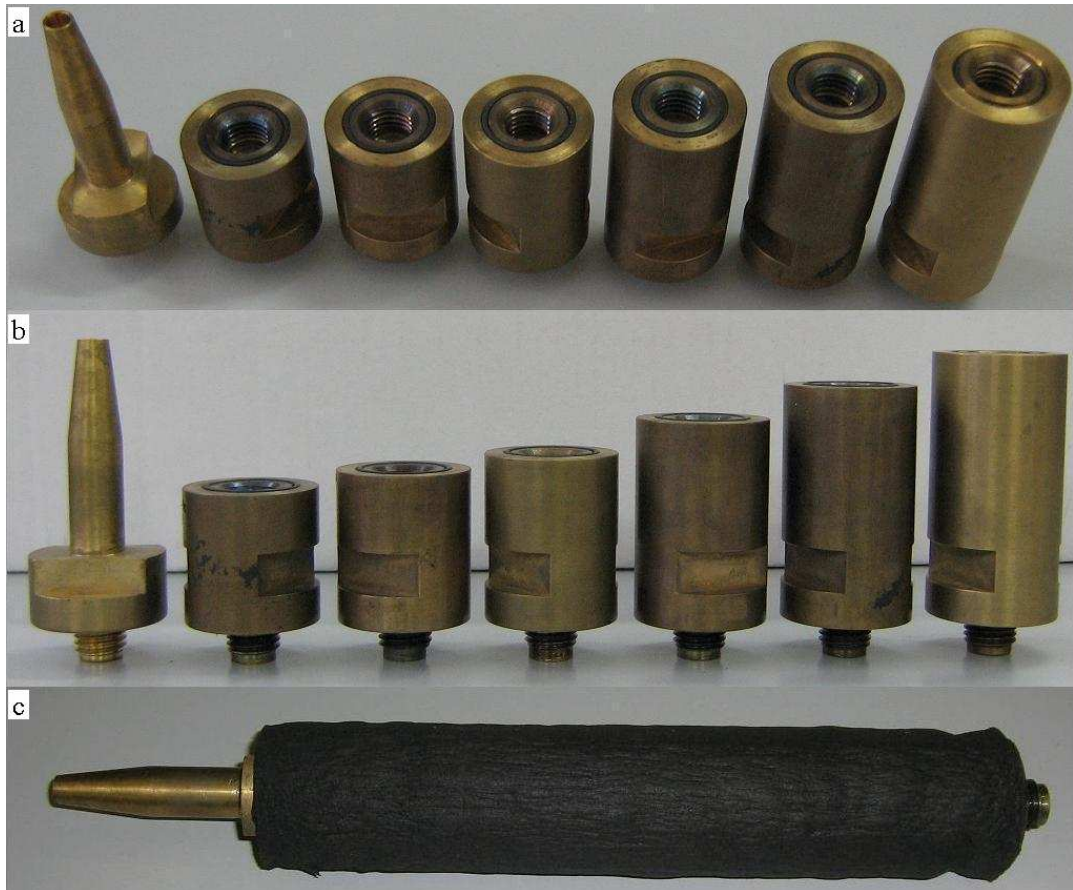
Figure 2.10: a,b) The nozzle and spacer c) The nozzle and spacers screwed together and covered with insulation
