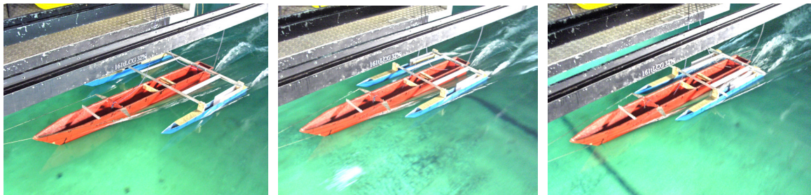
Figure F.14: Model at 4 m/s with 32 % LCG (From left to right: FOP, MOP and COP)
