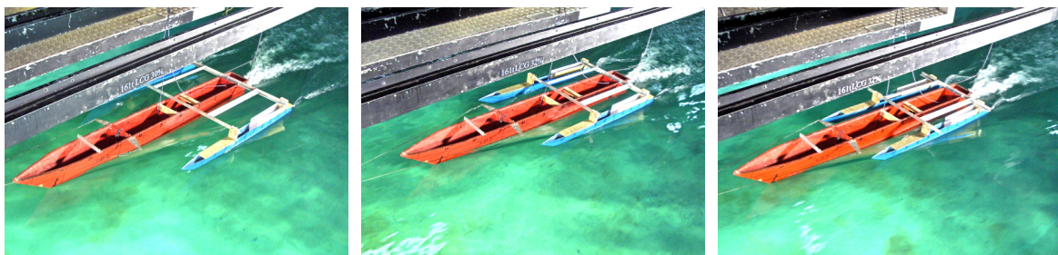
Figure F.16: Model at 2 m/s with 30 % LCG (From left to right: FOP, MOP and COP)
