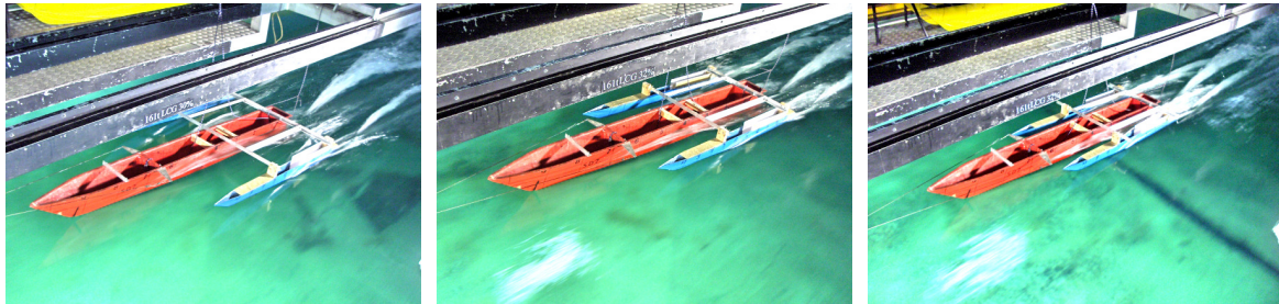
Figure F.18: Model at 6 m/s with 30 % LCG (From left to right: FOP, MOP and COP)
