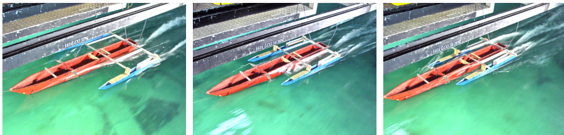
Figure F.12: Model at 6 m/s with 34 % LCG (From left to right: FOP, MOP and COP)
