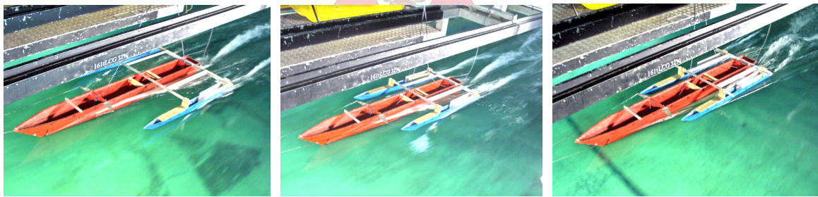
Figure F.15: Model at 6 m/s with 32 % LCG (From left to right: FOP, MOP and COP)
