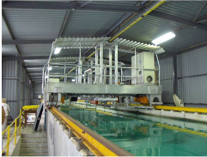
Figure 4.1: Towing tank and trolley
