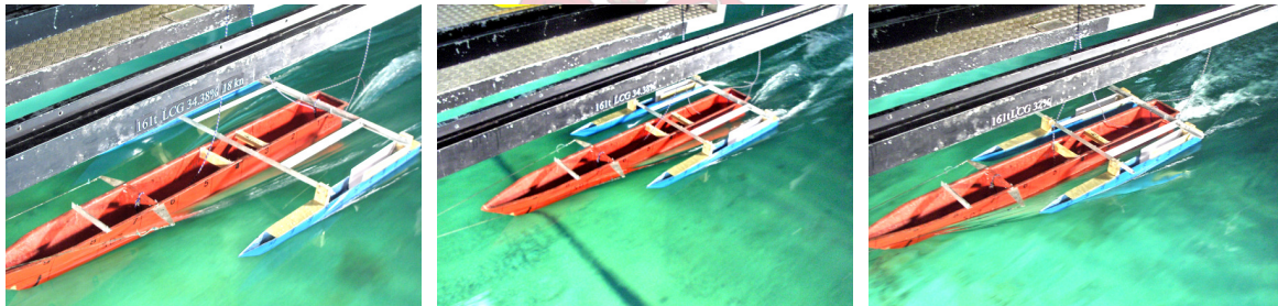
Figure F.11: Model at 4 m/s with 34 % LCG (From left to right: FOP, MOP and COP)
