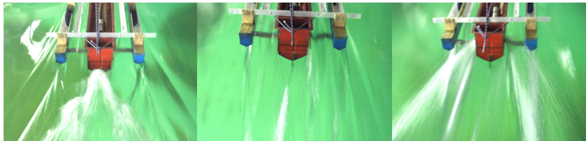
Figure F.20: Transom with 30 % LCG (From left to right: 2 m/s, 4 m/s and 6m/s)
