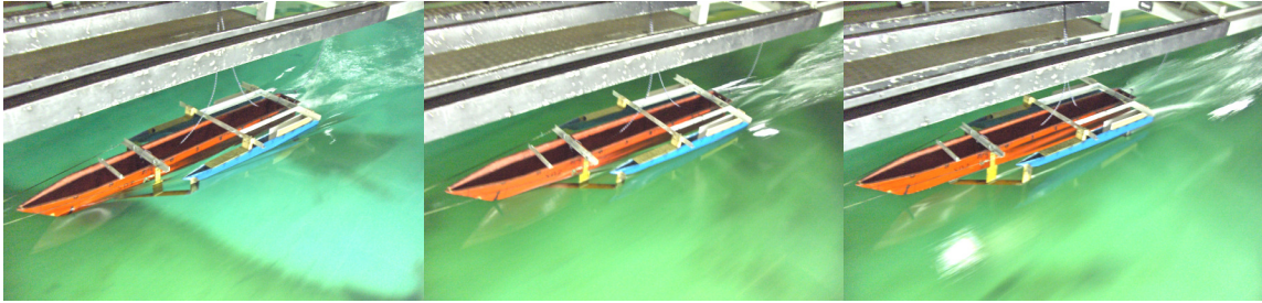
Figure F.21: Model with 32 % LCG (From left to right: 2 m/s, 4 m/s and 6m/s)
