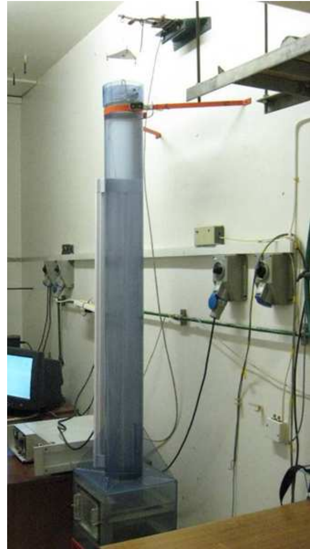
(b) Settling tube
