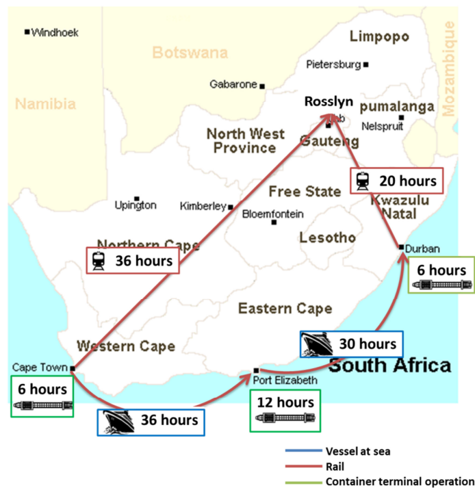
Figure 38 - Rail vs. sea and rail option for transporting BMW containers to Rosslyn
