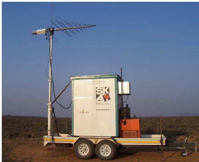
Figure 2-8: RFI Measurement System developed for the RFI Environmental Survey [1]
