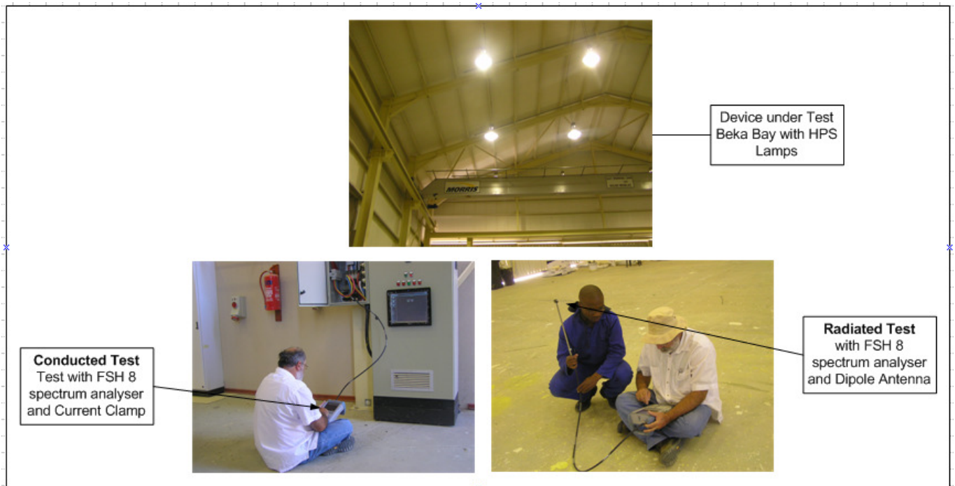
Figure 5-27: Test setup used at the Site Complex
