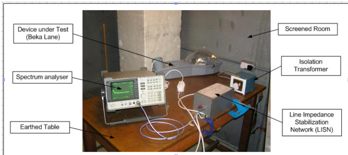
Figure 5-25: Test setup in the screened room at Stellenbosch University
