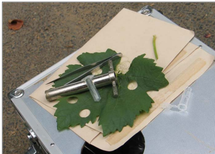
Figure 145 Image showing sampling positions on the leaf as well as instruments used during sampling.
