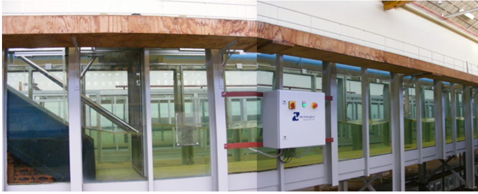
Figure 3.10: Wave flume creating waves
