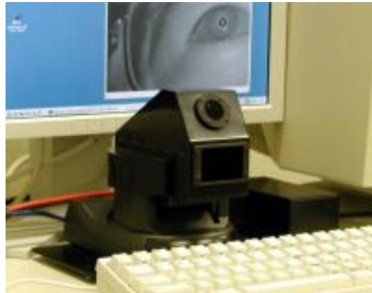
Figure 1.1: FreeGaze Gaze tracking system.
