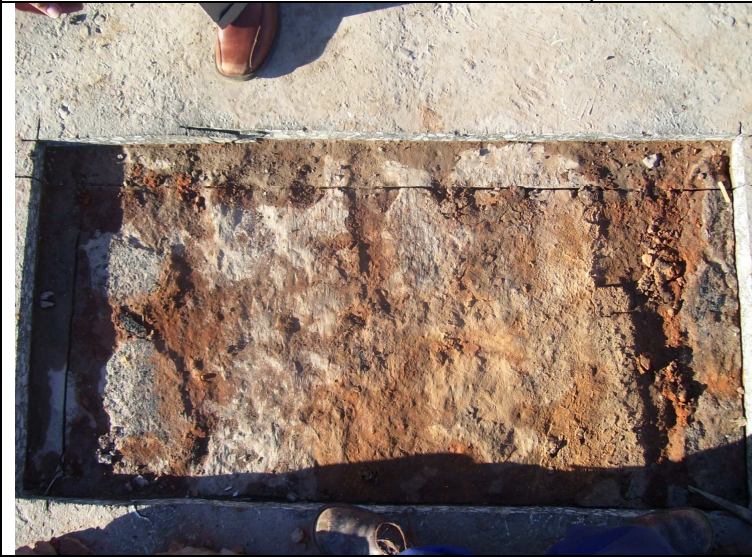
Plan and side view of CTB block. Note smoothed top surface.
