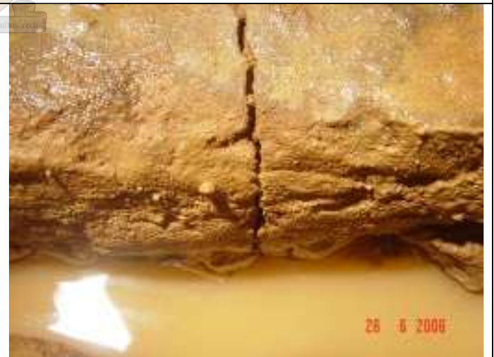
Longitudinal crack taken from the top side of the CTB block as well as side view
