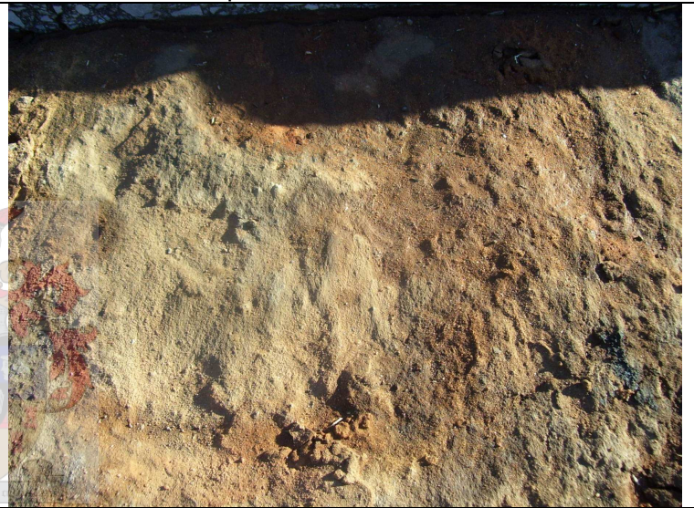
Pictorial overview of extraction. Plan view of CTB block. Note smoothed top surface.
