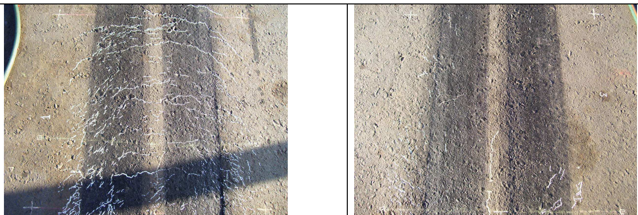
Plan view of sections after first 100 000 70 kN axles of traffic loading
