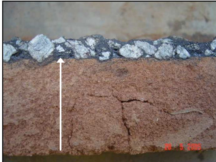
Figure 3.17e Close-up of 3 percent cement base with seal, shear plane on neutral axis of the 3 percent cement stabilized 50 mm scaled pavement clearly visible after 150 000 2.7 kN axle load repetitions
