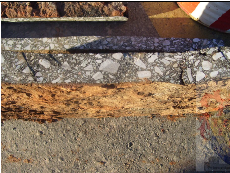
Side views of removed HMA mat note interface surfaces smoothed through shear fatigue
