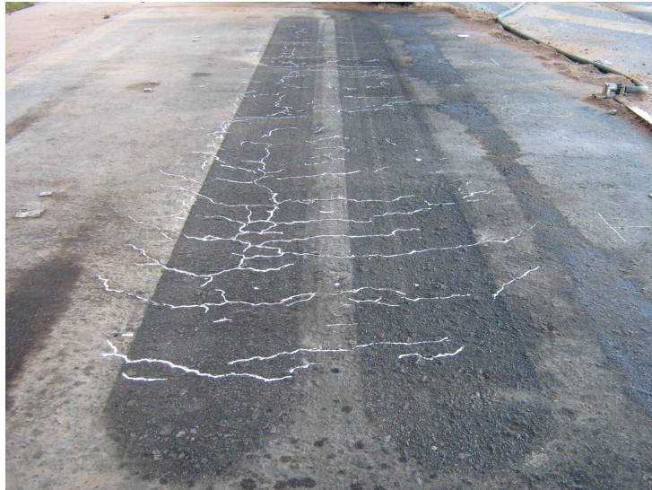
(e) Overview of Section 7 after 1 million 70 kN load applications
