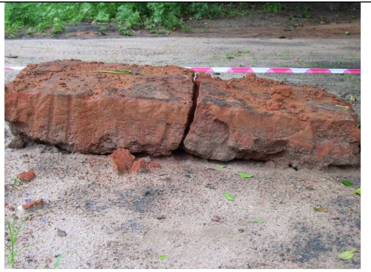
Removed CTB blocks from test pits 2 and 3. Note longitudinal cracks in direction of wheel travel and in plane shear cracking at the middle of the combined HMA and CTB structure.
