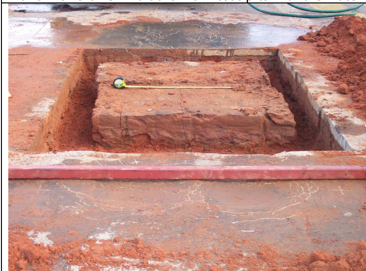
Pictorial overview of blocks and extraction of top part of CTB. Note mid layer shear plane intersecting with longitudinal and transverse cracks
