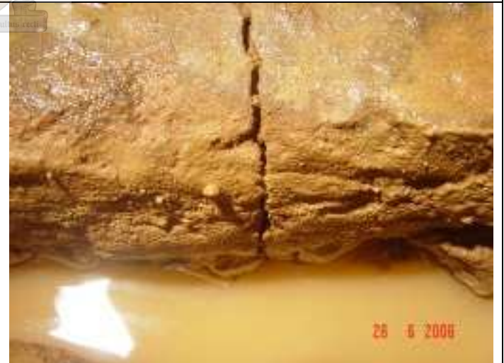
Longitudinal crack taken from the top side of the CTB block as well as side view
