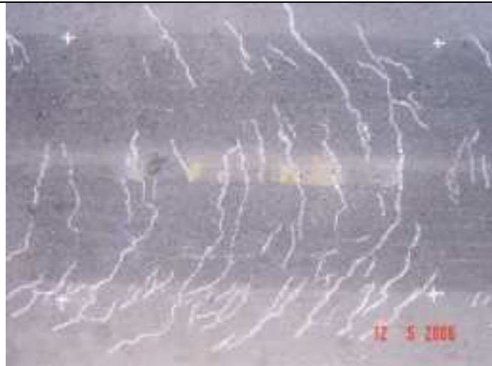
Plan views of test section with cracks drawn in with chalk
