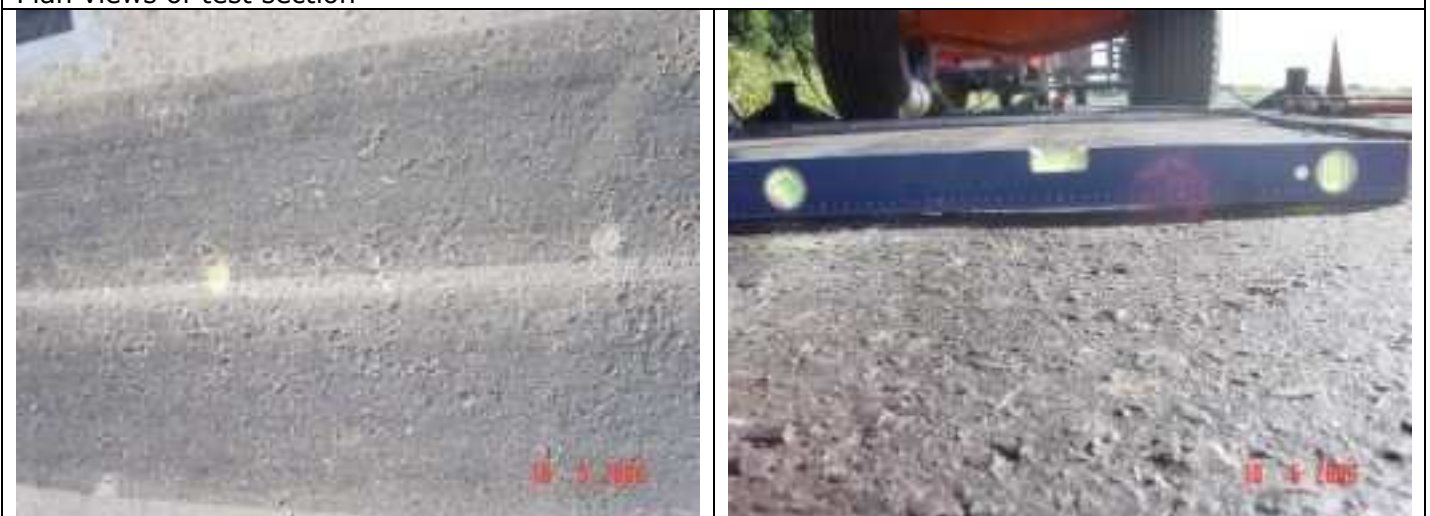
Plan view of test section and illustration of the extent of rut formation
