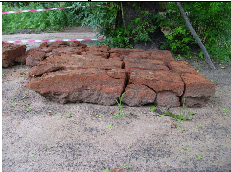
Removed CTB blocks from test pits 2 and 3. Note longitudinal cracks in direction of wheel travel and in plane shear cracking at the middle of the combined HMA and CTB structure.
