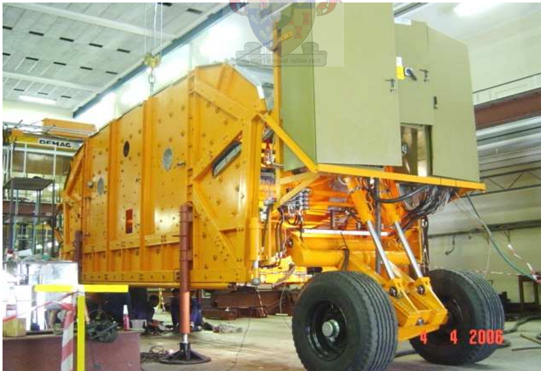
Figure 3.9: View of the MLS10 lifted in pavement monitoring and visual inspection configuration
