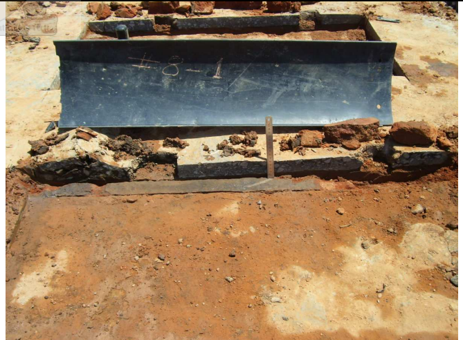
Underside of HMA mat after removal of test pit 3. Pictorial overview of all test pits with HMA removed.
