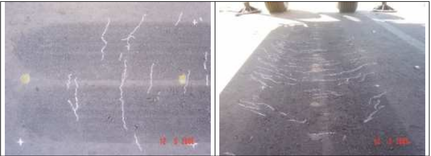
Plan and pictorial views of test section with cracks drawn in with chalk
