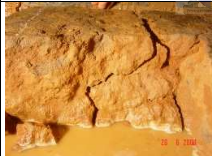
Pictorial views of marco cracks found in CTB block during extraction
