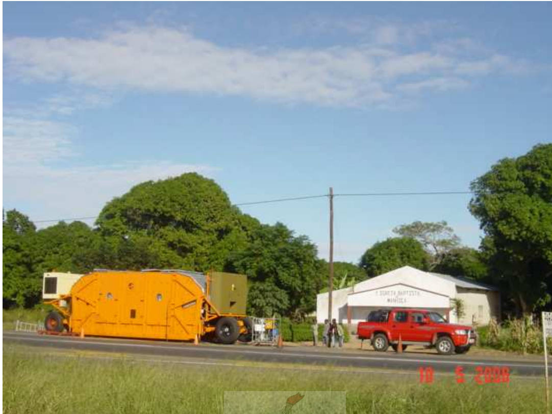
Figure 3.8: View of the MLS10 trafficking on the test site at Manhica in Mozambique
