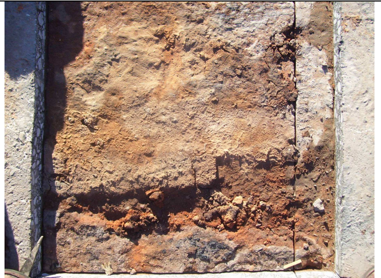
Pictorial overview of extraction. Plan view of CTB block. Note smoothed top surface.
