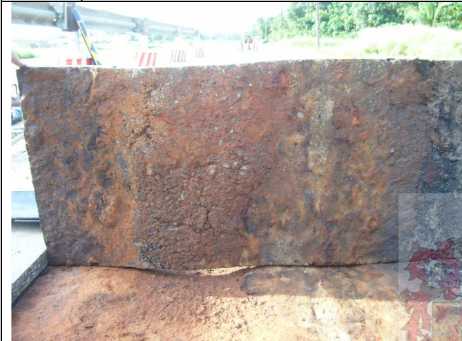
Underside of HMA mat after removal of test pit 3. Pictorial overview of all test pits with HMA removed.
