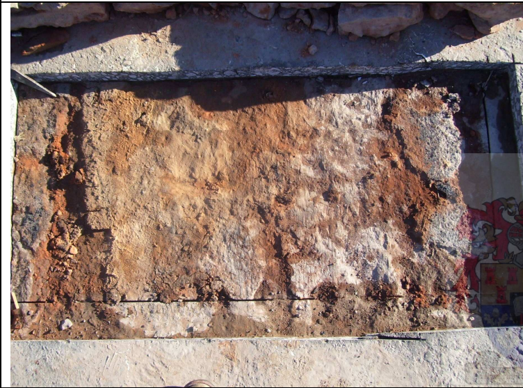
Plan view of CTB block. Note smoothed top surface.
