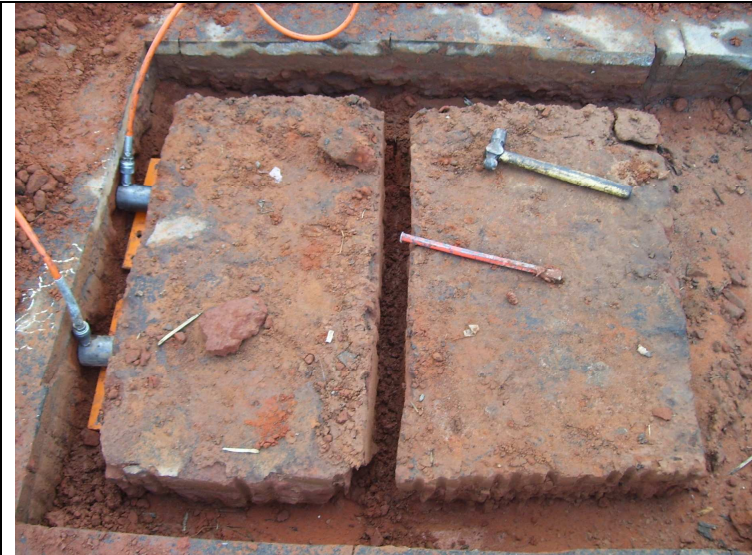
Pictorial overview of extraction. Plan view of CTB block. Note smoothed top surface.
