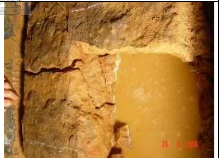
Pictorial views of marco cracks found in CTB block during extraction
