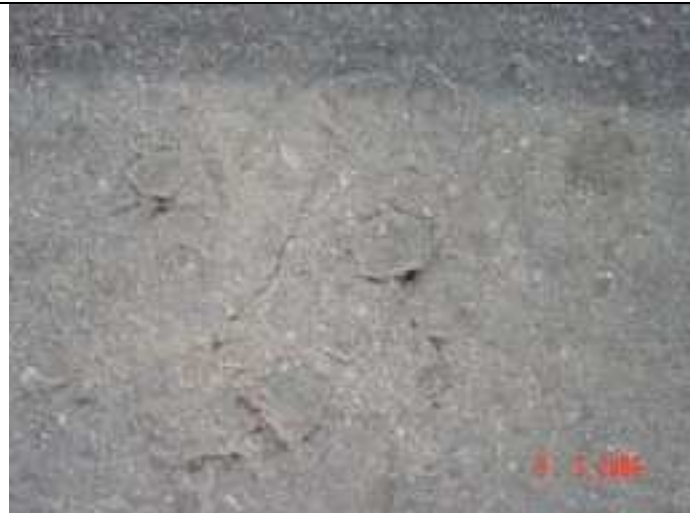
Surface crack initiation after 250 000 60 kN load applications
