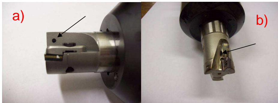
Figure 33: a) The customized toolholder for the PCD grades; b) The toolholder for the VP15TF
