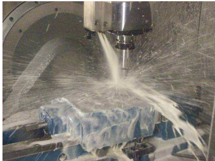
Figure 36: Flood lubrication supplied through the external nozzles.
