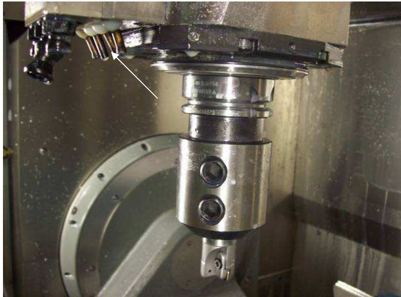
Figure 31: The external nozzles that direct coolant at the cutting zone for the flood lubrication experiments.
