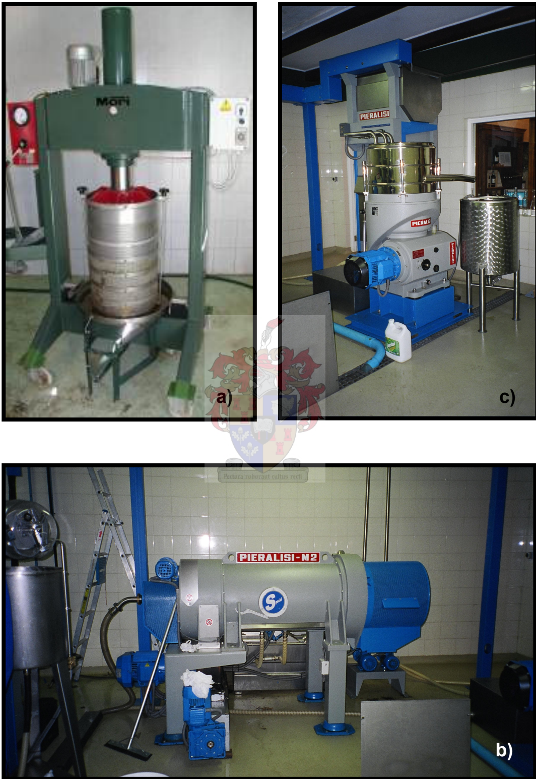
Figure 3 Photos depicting a) a hydraulic press, b) a centrifugal decanter or horizontal centrifuge and c) a separator or vertical centrifuge for the extraction and separation of extra virgin olive oil.
