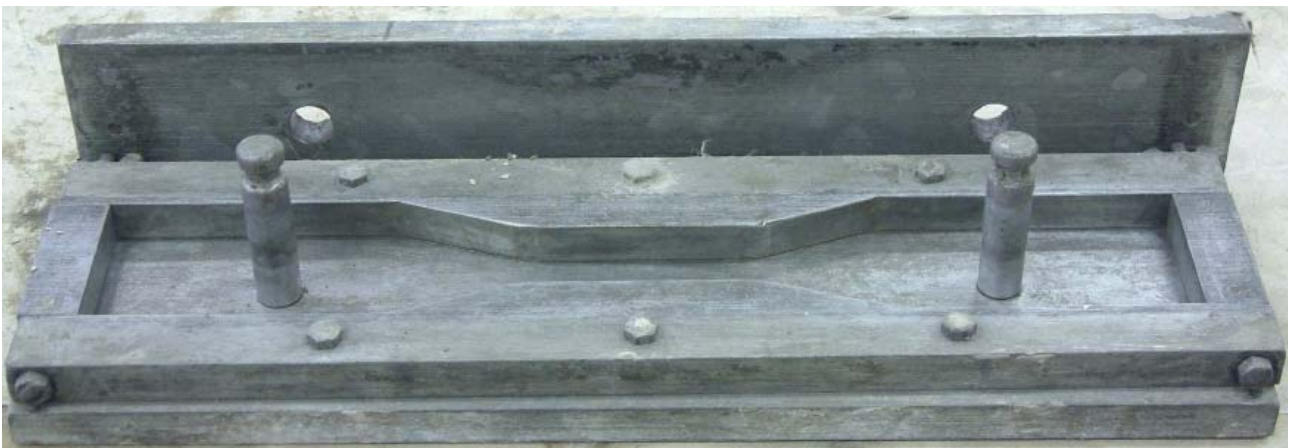
Figure 5.2: The steel mould used for casting of flat dog bone specimens with the two removable studs.
