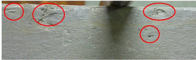
Figure 4.12: Surface flaws on extruded specimens.
