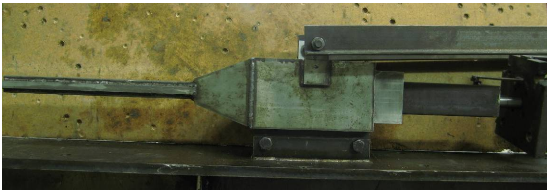
Figure 3.1: Piston-driven plate extruder developed by De Koker [2004].
