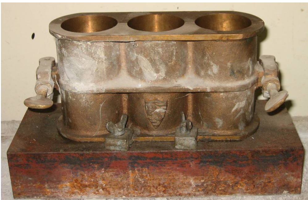
Figure 5.12: Copper mould used for casting SHCC cores.
