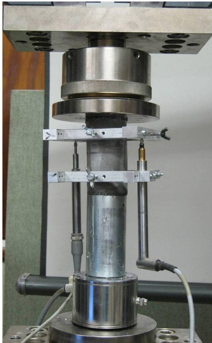
Figure 5.13: The compressive test set-up in the Zwick Z250 and the aluminium frame with the two LVDT's that were used to measure the strain over the gauge length.
