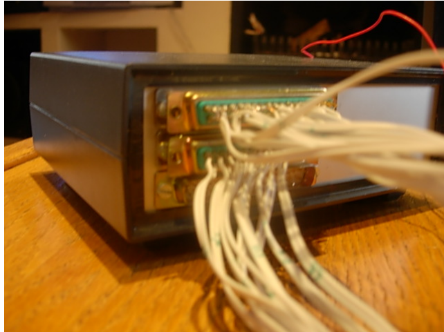
Figure 22: connection at the data acquisition box
