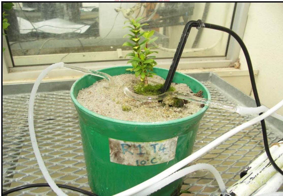
Plate 6.5 Cold water was pumped through glass spirals running through the pots to cool down the root zone.
