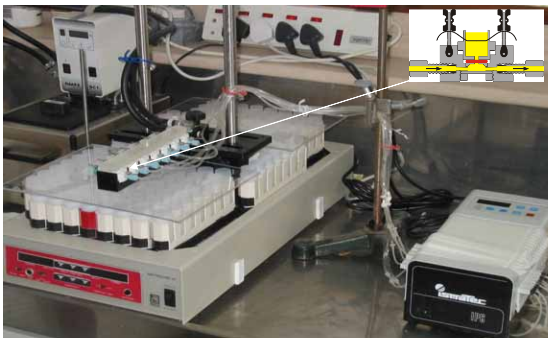
Figure 6. Flow-through diffusion apparatus used in the present study.
