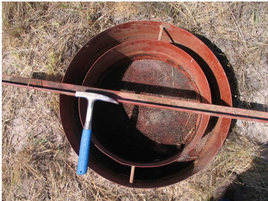
Figure 3.3: Photo of double ring infiltrometer used during infiltration experiments.
