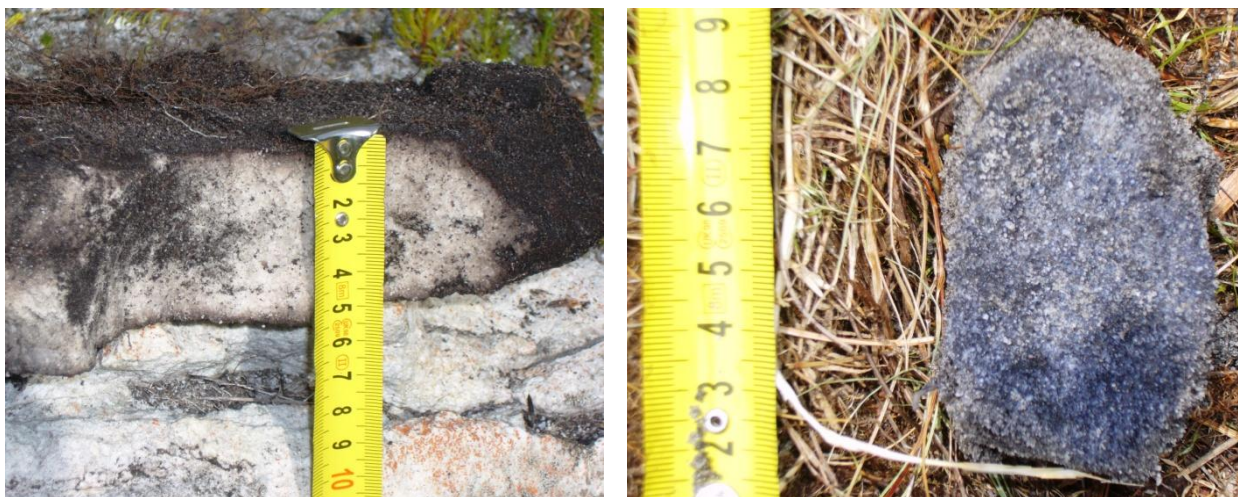
Figure 3.10: Table mountain sandstone removed from profile K1: Left: No blue colour formation indicating antecedent moisture only. Right: Blue colour formation indicating infiltration of KI solution overnight.
