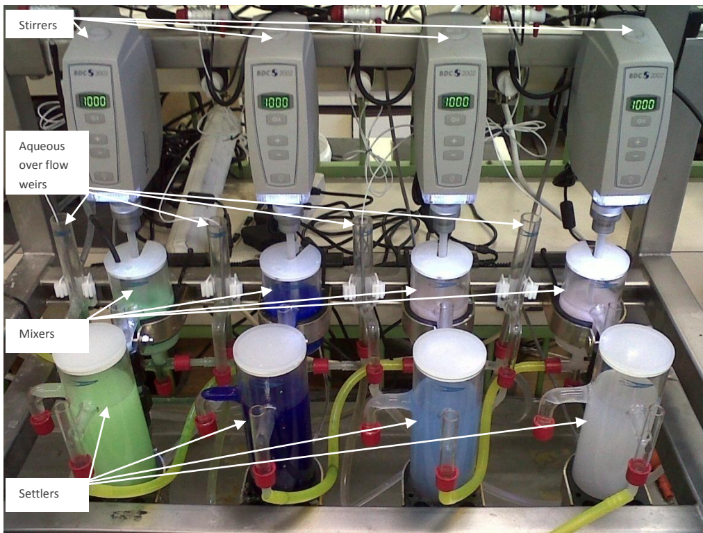
Figure A-8: Photograph of the agitators, mixers, settlers and aqueous overflow weirs
