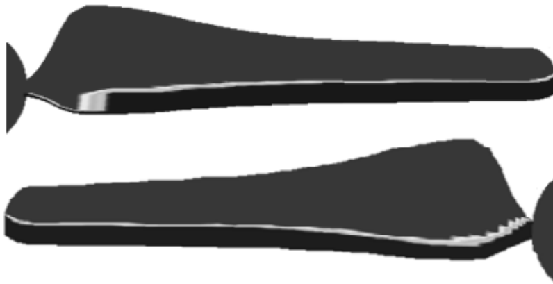
Figure 45: Intermittency plot of wind turbine rotor as seen from upstream (top) and downstream (bottom)
