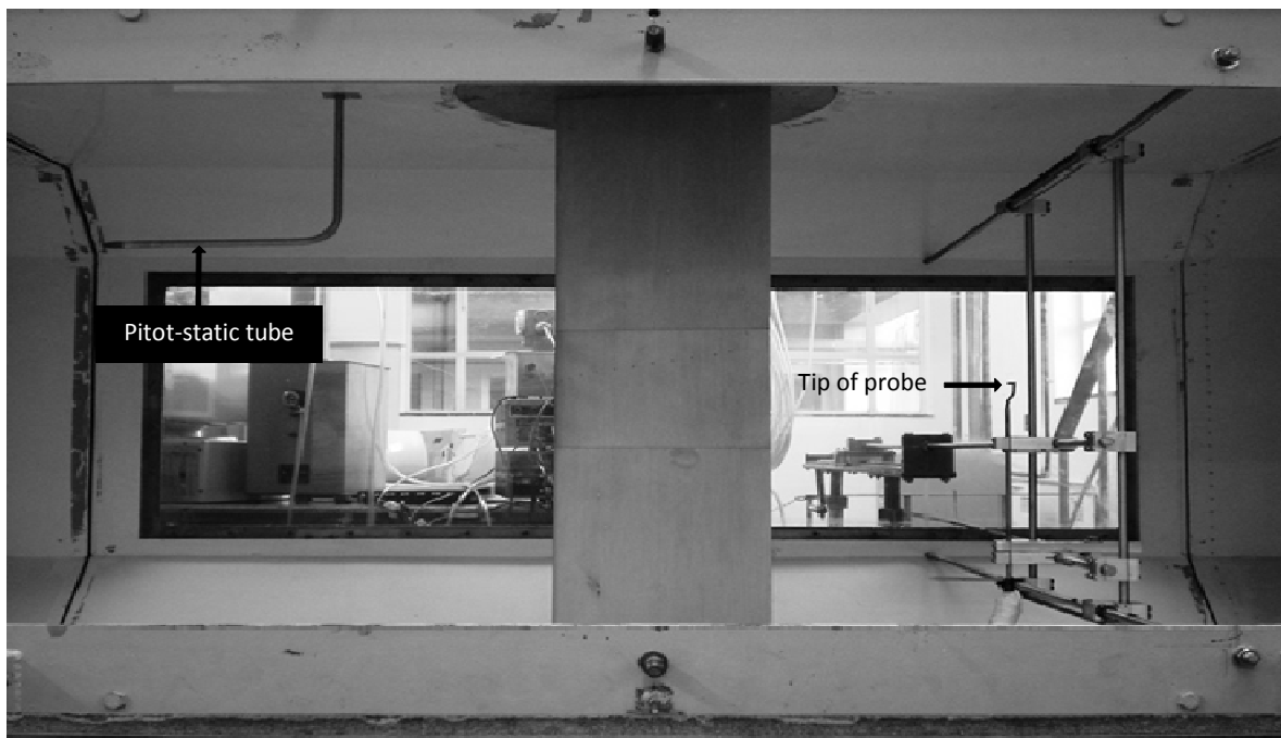
Figure 13: Model mounted in wind tunnel test section.
