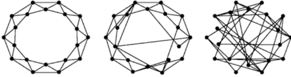
Figure 3.1: The initial configuration for the Watts and Strogatz model with n = 20 and k = 4 (left); the resulting network for some 0 < \beta < 1 (middle); and the resulting network for \beta \approx 1 (right). Diagram reproduced from [22].
