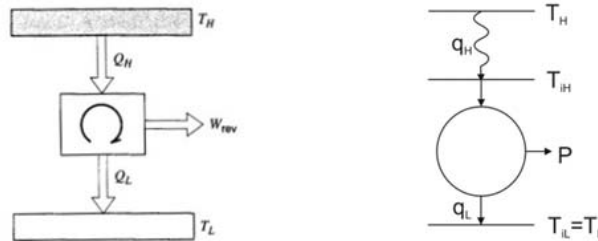
Figure 29: Reversible heat engine cycle (left) (van Wylen, Sonntag & Borgnakke 1994) and Novikov engine as reversible Carnot engine, with irreversible link to heat source T_H (right) (Wagner 2008)
