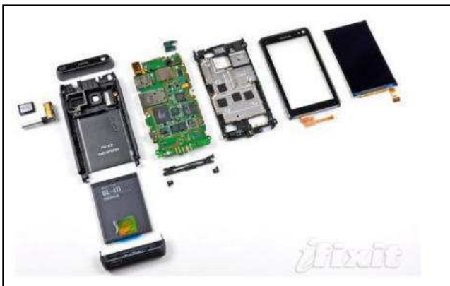
Figure 4: Mobile phone components (Our Nokia, 2011)
