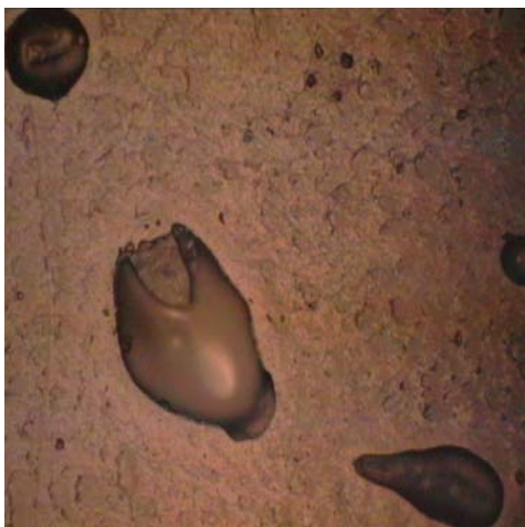
Figure 5.37: Surface erosion in PDMS sample C caused by acid rain ageing, observed after 75 days.
