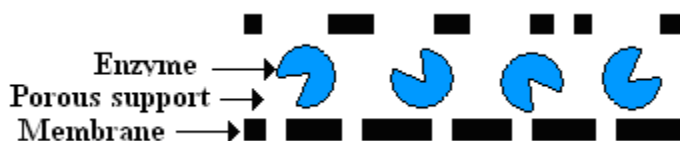
Figure 2.6: Immobilisation through physical adsorption in membrane pores
