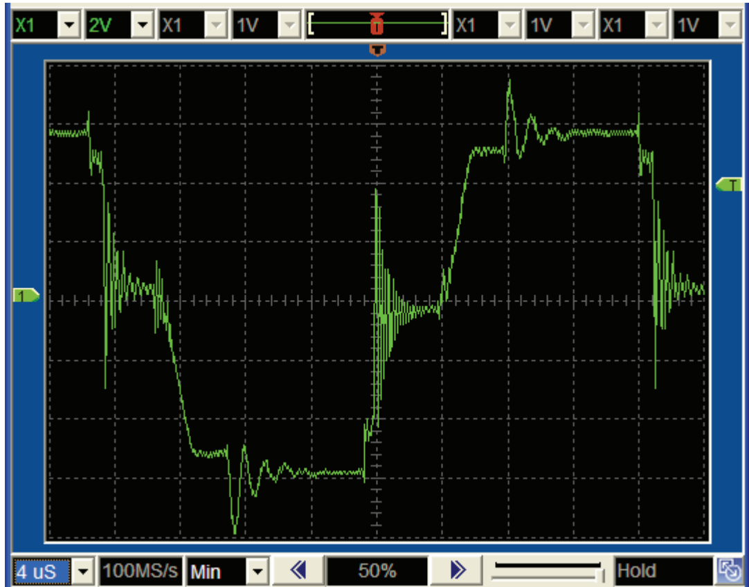
Figure 70: Reverse Mode, Rectifier Input Voltage (Ch.1)
