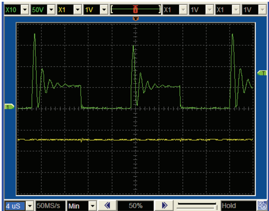
Figure 68: Rev. Mode, Pos. Input, Inductor Voltage (Ch.1) and Current (Ch.2)
