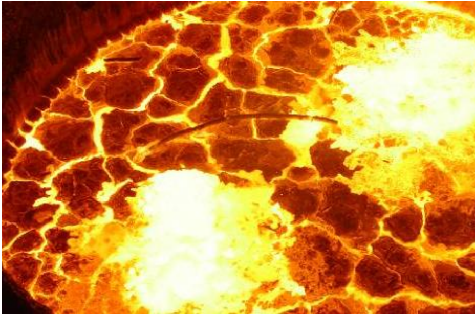
Figure 63: Plume eye formation in the actual ladle at 0.00267 kg/s/plug.
