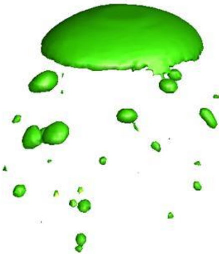
Figure 81: Large bubble surrounded by smaller bubble fragments continuously breaking away and rejoining.
