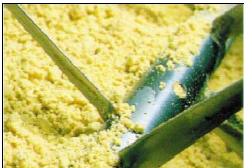
FIGURE 2.2 CORRECTLY HYDRATED SEMOLINA (MONDELLI, 2002:16)
