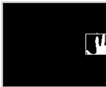
Figure 32. The small width of the white object determines controlling movement, but the hand is open. Also, the position determined for the hand is not the centre of the hand.
