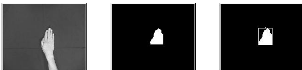
Figure 20. After mirroring and after splitting (closed hand), bounding rectangle.
