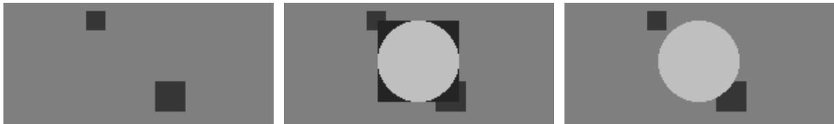
Figure 22. Illustrating transparency with first a background image, a circle image added and then a circle image with transparent regions added instead.
