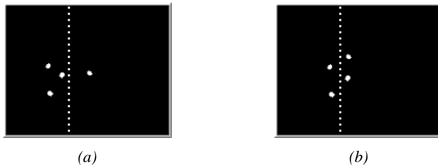
Figure 33. In (a) the dotted line represents the image split by separating left from right hand. It is incorrect as the right thumb is grouped with the left fingers and controlling movement is determined for the right hand. In (b) a solution is provided when hands are close together.
