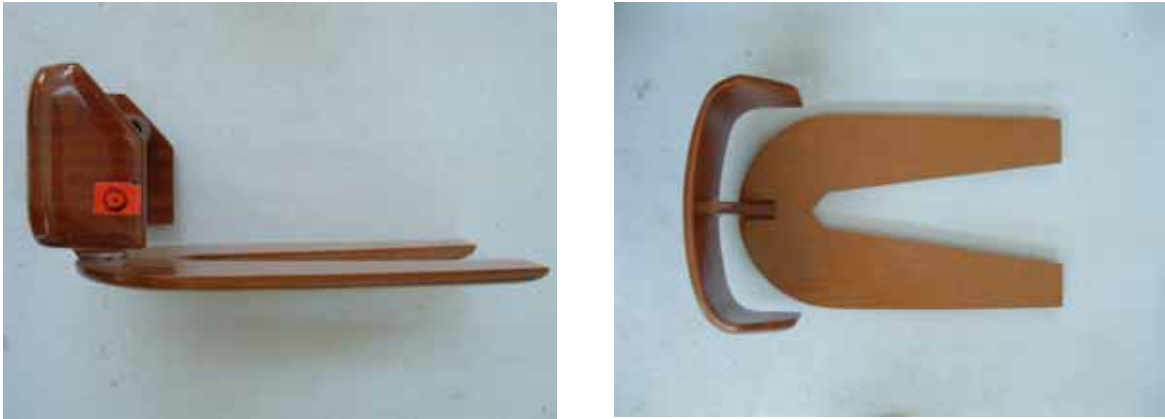
Figure 2.3 A seat index point (SIP) gauge
