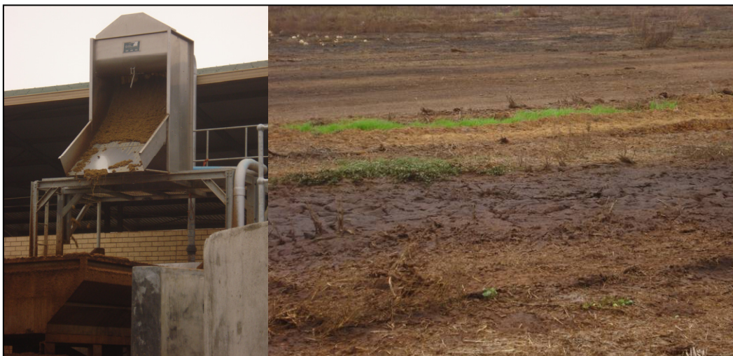
Figure 4.20: Vyevelei system, showing a static screen separator and manure trailer, and smothering caused by the incorrect method of applying dairy waste to land.
