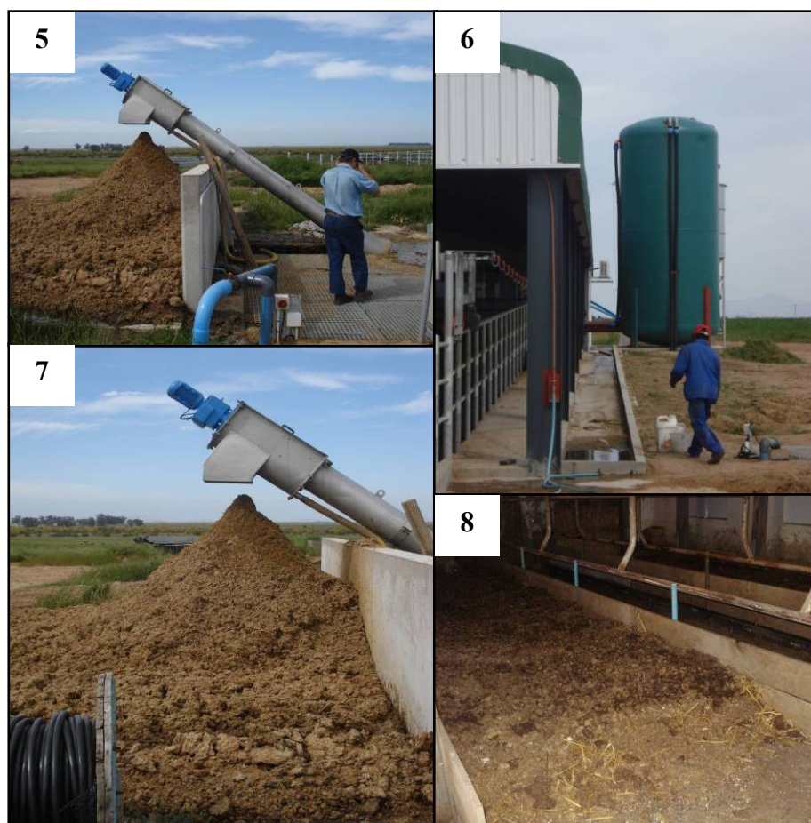
Figure 4.23: Uilenkraal dairy system, showing the use of a screw auger separator, recycled water storage for the wash down of holding area, the separated solids, and the new worm farm that is used in composting procedures.
