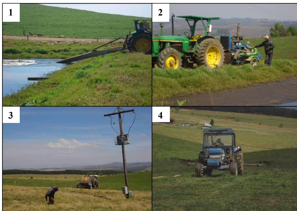
Figure 4.14: Denleigh Farm system, showing agitation of slurry and subsequent application to pastures via umbilical pipes and a tractor mounted dribble bar.
