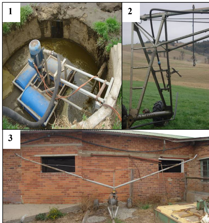
Figure 4.18: Mearns Farm system, showing agitation of slurry and subsequent application to pastures via both a pivot mounted gun applicator, as well as a traveling gun applicator.
