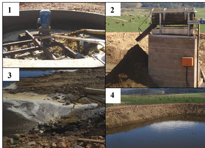
Figure 4.11: Ericsberg Farm system, showing separation of slurry using a rotary screen system and storage of liquid waste in a storage lagoon.
