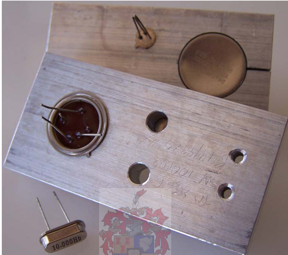
Figure 3.12: Photograph of the different quartz crystal resonators that were used in oscillators for this project. The low profile crystal to the front left is a commonly available AT-cut crystal while the other two crystals are of SC-cut (crystal in centre is contained in an HC-37/U package; crystal at back is contained in HC-40/U package) and are shown here in aluminium blocks which act as heat tanks that are also fitted with temperature sensors.
