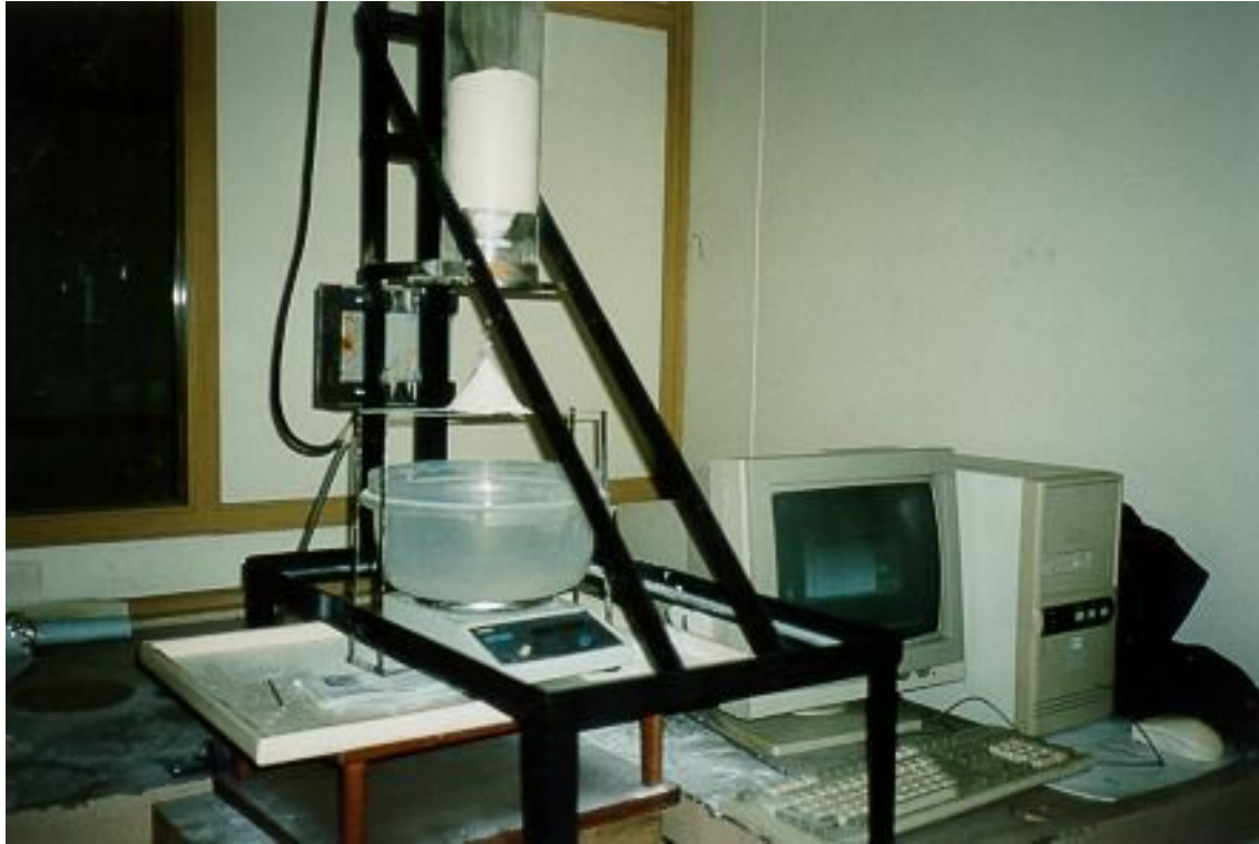
Figure 7.9 Experimental set-up used to investigate avalanching behaviour of various types of particles.
