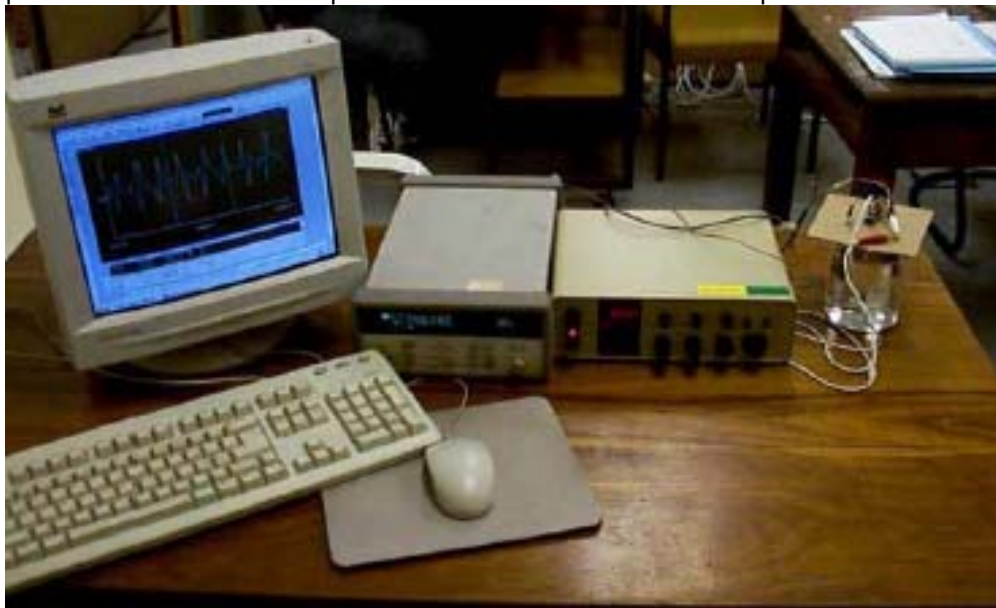
Figure 5.9 Experimental set-up used to measure electrochemical noise data.
