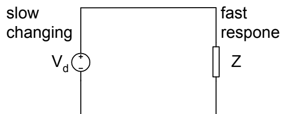
Figure 5-1. Basic circuit with slow changing source.
