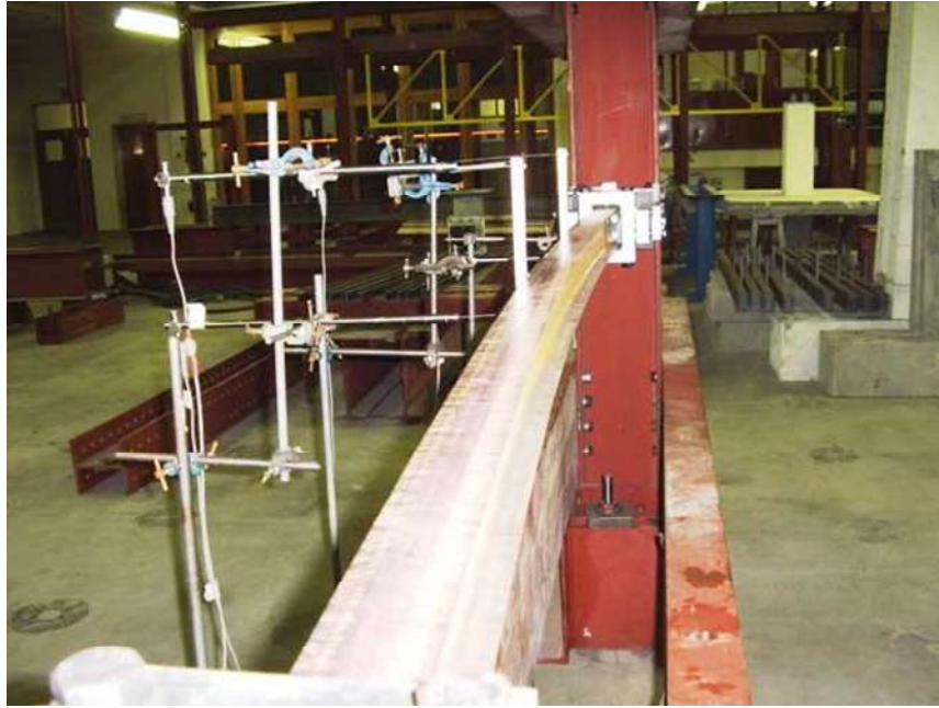
Figure 4.19 - Buckled shape of Test 1
