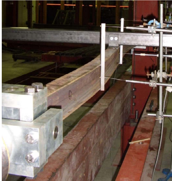
Figure 4.20 - Buckled configuration of Test 4
