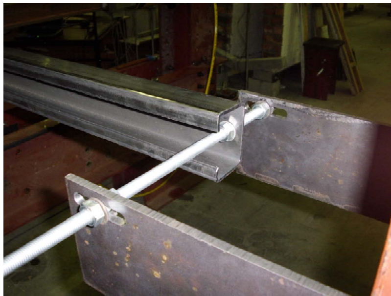
Figure 4.10 - Sheeting rail boundary condition
