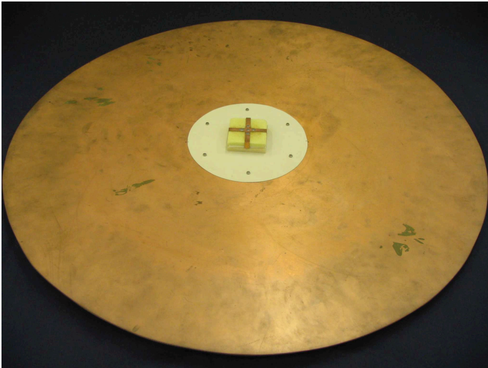
Figure 5.6: Antenna with conductive ground plane.
