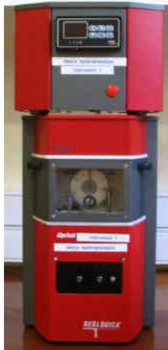
Figure 1. The rigometer (Rigotech®) is used to measure isometric tension ( \text{mN}\cdot\text{mm}^{-2} ) and shortening (%) during the development of rigor mortis in the muscle strips at constant temperature ( ^{\circ}\text{C} ).
