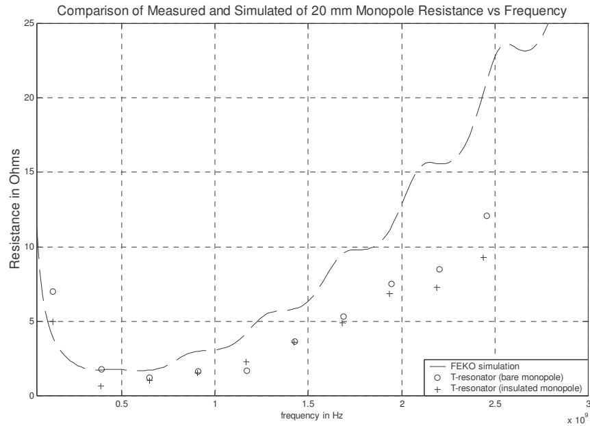
Fig.3.4 Comparison between measured and simulated results of the 20 mm monopole resistance
