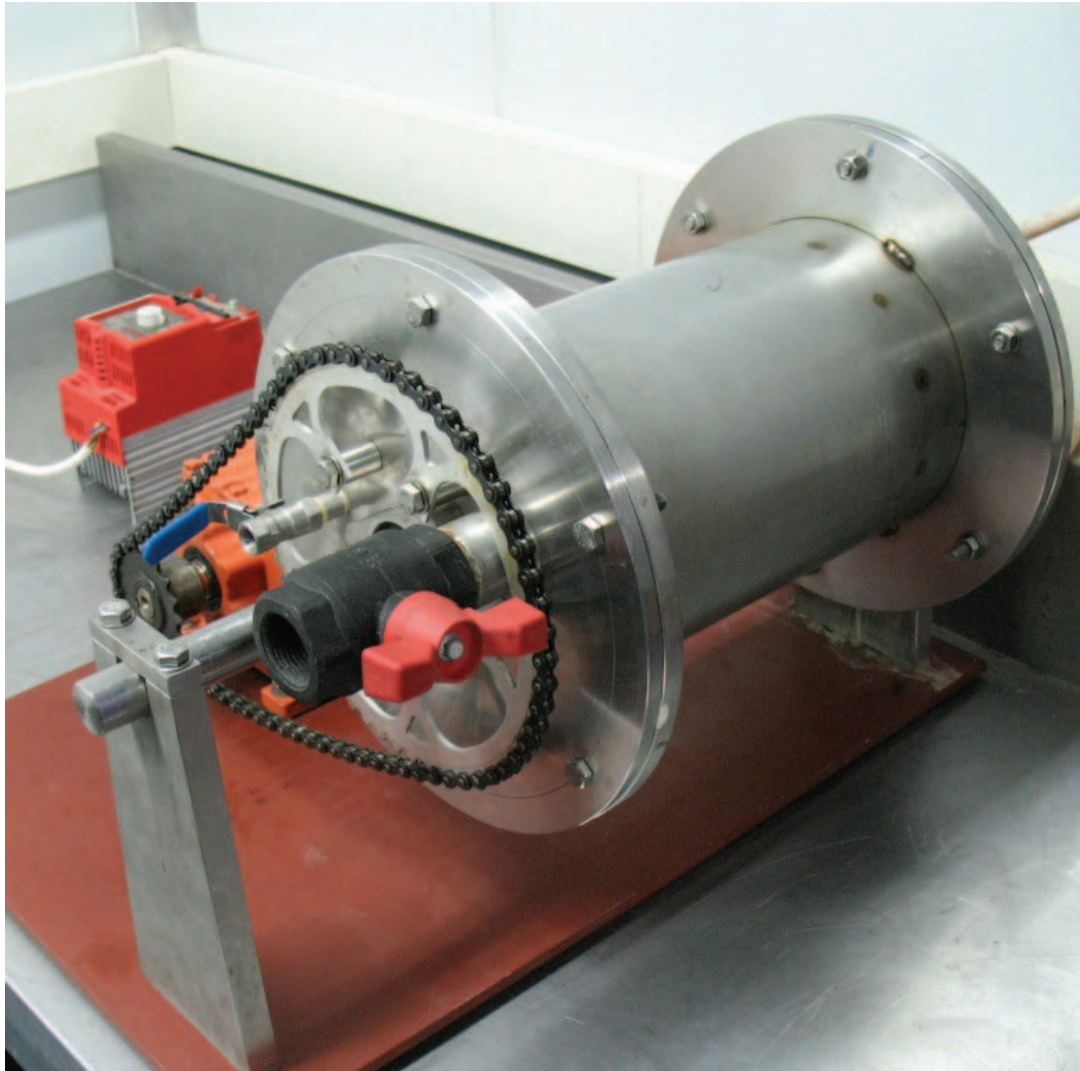
Figure 1 Cylindrical reactor used in this study for the pre-treatment of the UASB reactor inocula for reactors B and C.
