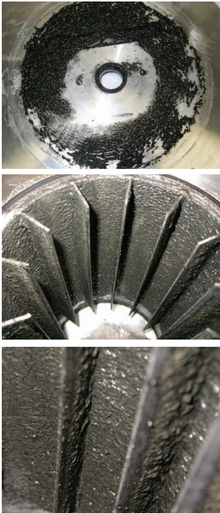
Figure 5 Biofilm formation observed on the inside of the rolling batch reactor after batch granulation-enhancement batch 7.
