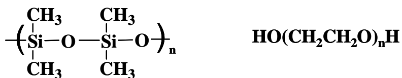
Figure 1. Chemical structures of two of the widely used stationary phases in CGC: apolar polydimethylsiloxane (PDMS, left) and polar polyethylene glycol (PEG or wax, right).
