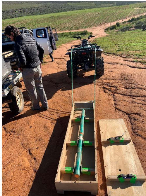
Figure 2.4: A DF Instrumental CX Mini Explorer 2, attached to a quad bike, used to measure electrical conductivity during the electromagnetic induction survey.
