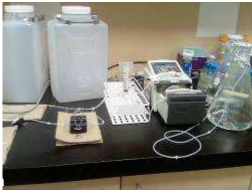
Figure 3.5 Flowcell design for developing biofilms (a) Flowcell setup with fresh media continuously being pumped through the flowcell by means of a peristaltic pump, to the outflow of waste on the left. (b) Perspex flowcell containing a 25mm x 4mm x 6mm chamber, sealed with glass microscopic slides on either side.
