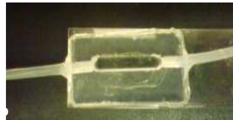
Figure 3.5 Flowcell design for developing biofilms (a) Flowcell setup with fresh media continuously being pumped through the flowcell by means of a peristaltic pump, to the outflow of waste on the left. (b) Perspex flowcell containing a 25mm x 4mm x 6mm chamber, sealed with glass microscopic slides on either side.
